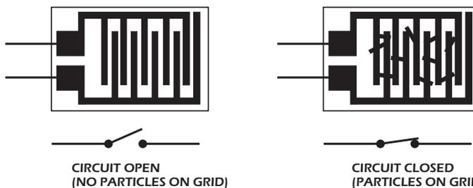
Activation of the MPD switch occurs when metal particles bridge the gaps on its electrical grid and complete a normally open (N.O.) electrical circuit to drive an alarm or shutdown relay (refer to Figure 2).
