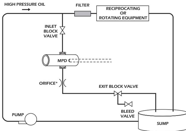
Operation is simple and straight forward. Process fluid, such as lube oil or transmission fluid, enters at the top of the MPD's body. Fluid then travels through a perforated board containing a plated electrical grid on the board's top and bottom sides. Fluid exits through the bottom of the MPD body (refer to Figure 1).
